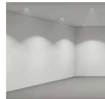
Extra wide flood light distribution Light distribution with an emission angle of 90° and a 40° cut-off for uniform lighting with high cylindrical illuminances.
